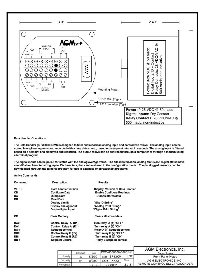
To access the configuration: First start either the SCADA.EXE program shipped with your Super Puk, or you may use your own terminal emulator program. You may use any terminal program that supports standard ASCII. Set the communications parameters to no parity, 8 data bits and one stop. Baud rates may be either 300, 1200, or 9600 baud.
