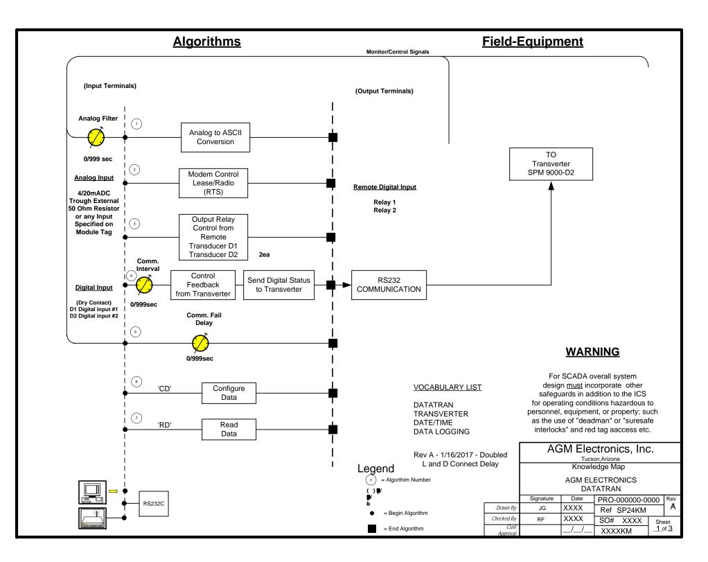
To Access the super puk configuration, type 'SCADA" from the drive/directory installed with the software provided in this shipment. You can use any terminal program that supports serial ASCII communications and use the same active commands. The terminal program provided herewith contains help notes on the super puk configurations. This program defaults to serial port COM:1.
